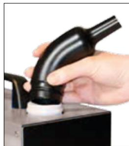
3. Connect the specific conveyor tube to *Ultrasound Clean Machine*.
