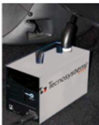
1. Start engine and place *Ultrasound Clean Machine* on the floor mat at the passenger side and set the conveyor tube as much closer as possible to the ricirculation air intake.
