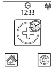
The pump will activate and the disinfectant soon begins to circulate. After 4 minutes, the pump stops for about 20 minutes and then restarts for a further minute. After this time, a symbol appears on the display to indicate that the bath is ready to be emptied.
